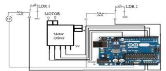
Fig.3. Microcontroller based solar tracking circuit for PTC
