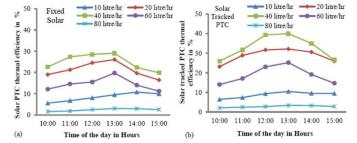
Fig.6. Solar PTC thermal efficiency plot for different flow rates
