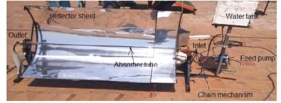
Fig.5. Solar Parabolic Trough Collector
