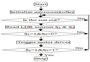
Fig.4. Solar tracking control algorithm
