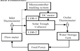
Fig.1. Schematic of single axis parabolic trough collector
