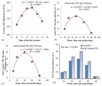
Fig.7.(a) Correlation between time of the day and average solar radiation; (b) Correlation between water flow rate and static PTC thermal efficiency; (c) Correlation between water flow rate and solar tracked PTC thermal efficiency; (d) Solar PTC thermal efficiency plot for different flow rates
